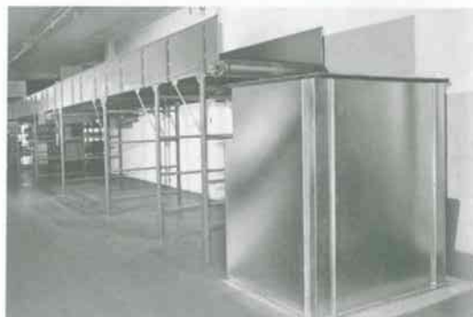
Central conveyor dumps boxes and scrap into large hopper for automatic shredding, baling or compacting.
